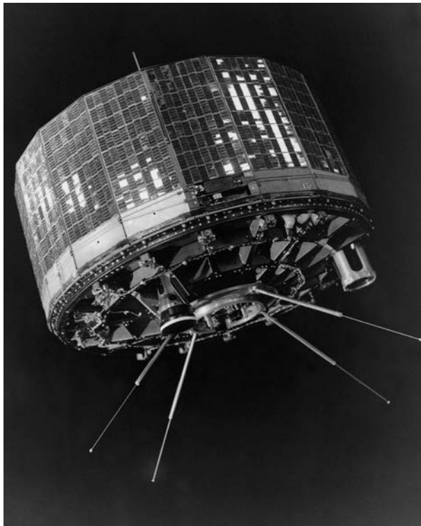
[Figure 2] TIROS program weather satellite, 1970. The TIROS Program (Television Infrared Observation Satellite) was NASA's first experimental step to determine if satellites could be useful in the study of the Earth. At that time, the effectiveness of satellite observations was still unproven. Since satellites were a new technology, the TIROS Program also tested various design issues for spacecraft: instruments, data and operational parameters.
