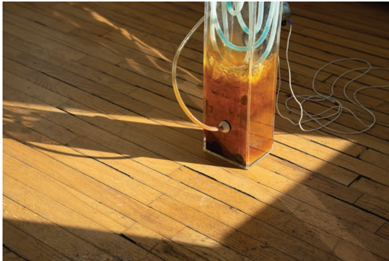
[Figure 4] Cemented copper and iron in the bottom of Accumulator 01.
